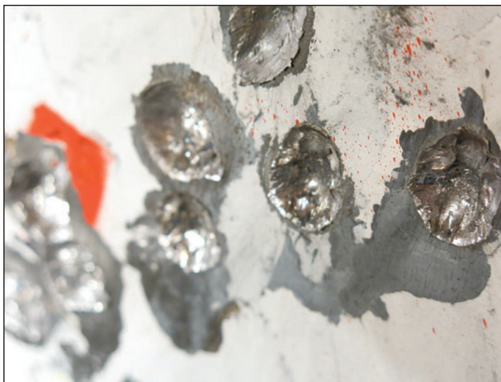
Figure 10 —Cratering of AR-500 steel plate by steel core bullets was visible at high impact angle (60-80 degrees from horizontal) but not at low angles (20-40 degrees from horizontal).
