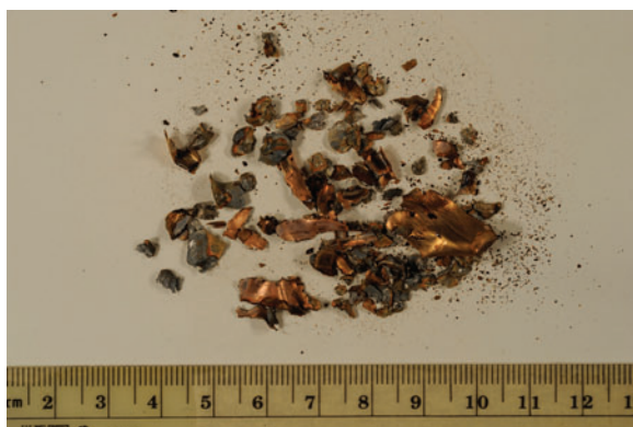
b) 7.62x51, 150gr, Lead Core, Copper Jacket FMJ
